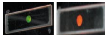
Figure 5. Colours of a 7.4% w/w solution of the EE isomer of ( R )- 1 in ZLI-2359 (left) and of the visible photostationary state (right).
